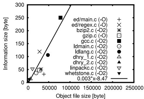
**Fig. 5** Information density by reordering instructions in each basic block.
