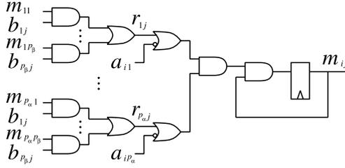
Fig. 3 Element circuit for refinement procedure.
