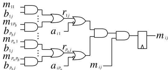
Fig. 2 Element circuit for refinement procedure.
