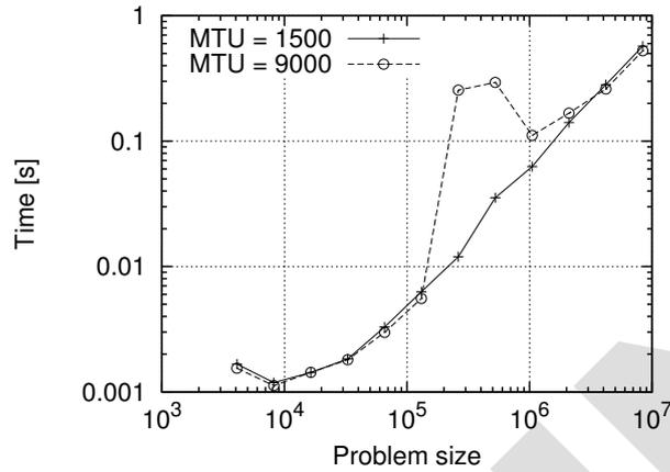
Figure 23. The execution time of FFTE among 16 Xeon processors: MTU=1500 and MTU=9000.
