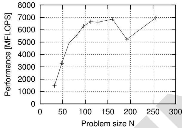
Figure 8. An example of measured performance of Himeno benchmark, where a performance anomaly exists at  $N = 192$ .
