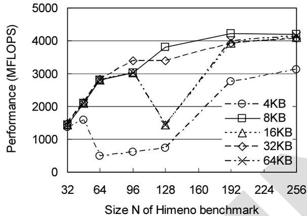
Figure 27. Sensitivity of Himeno benchmark performance to the buffer size of MPI library. Measurements made with 16 Xeon processors.
