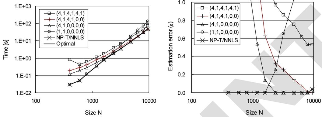
Figure 15. Comparison of various process allocation schemes for HPL benchmark. Left graph displays the execution time of the actual optimal configuration (Optimal) and those of estimated optimal configurations by various allocation schemes. Right graph displays the corresponding estimation error ( $\epsilon$ ).
