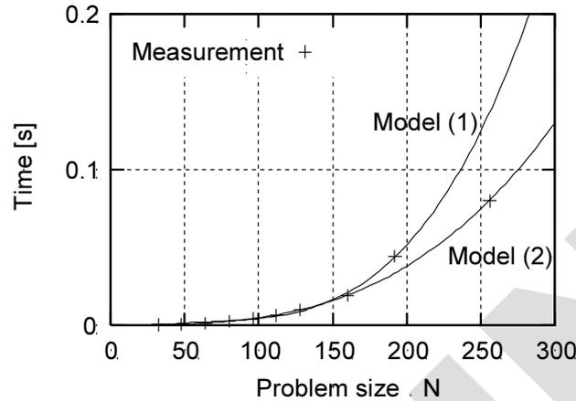
Figure 9. Performance anomalies affect the model parameters extracted. Model (1) was extracted from all measurement results, while Model (2) was extracted from the measurements excluding  $N = 192$ .
