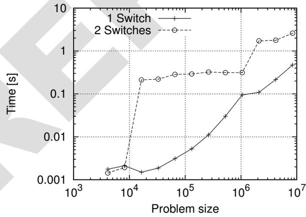
Figure 26. The execution time of FFTE for two network topologies.
