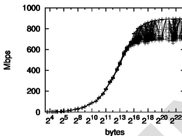
Figure 28. Network transfer rates between Pentium 4 and Athlon 64 X2 with Cool'n'Quiet feature enabled. Figure displays the results of 144 trials, which are quite unstable and unpredictable.
