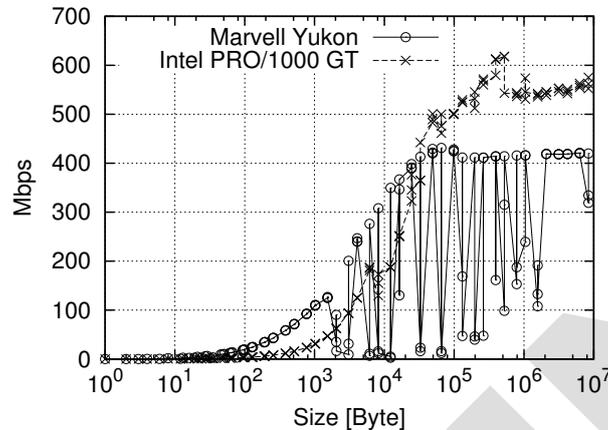
Figure 21. Network transfer rates of Marvell Yukon and Intel Pro/1000GT network interfaces.
