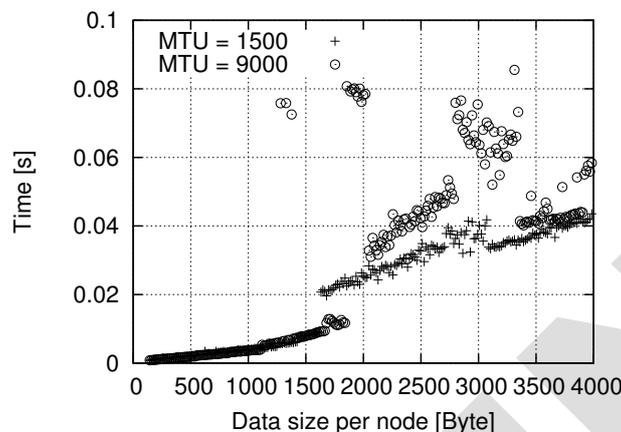
Figure 22. Latencies of all-to-all communication among 16 Xeon processors: MTU=1500 and MTU=9000.
