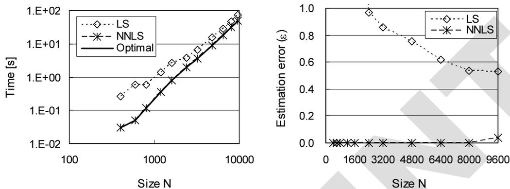
Figure 13. Parameter extraction for NP-T model by least squares method (LS) and non-negative least squares method (NNLS) for HPL benchmark. Left graph displays the execution time of actual optimal configuration (Optimal) and those of estimated optimal configurations with the parameters extracted by LS method and NNLS method. Right graph displays the corresponding estimation error ( $\epsilon$ ).
