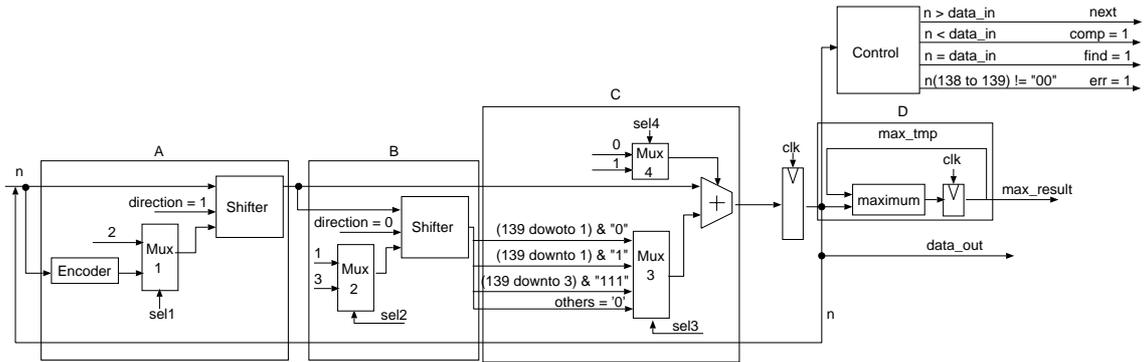
Fig. 3. Block diagram of CP2/S8/A1/NMX.
