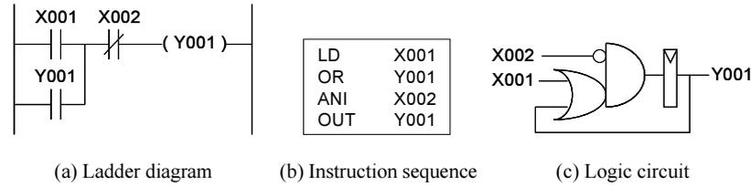
Fig. 2. An example of FX2N PLC program: self-holding logic. <sup>(3)</sup> (©2006 IEEE)
