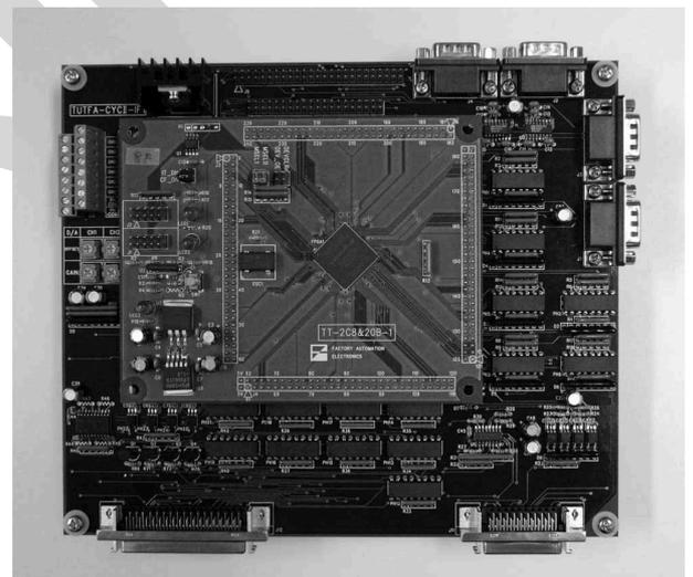
Fig. 10. TUTFA-CYCII-FI: an FPGA control board with an Altera Cyclone II device and various I/O channels.
