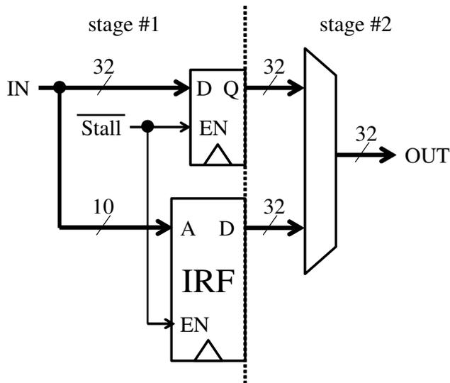
Figure 13: An implementation of the IRF, where the output of the IRF is passed to the decoder when a specialized instruction is fetched.
