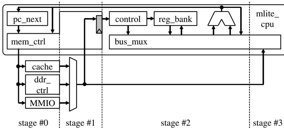
Figure 12: The *two-stage* pipeline of the Plasma processor [23], whose actual number of pipeline stage is four.
