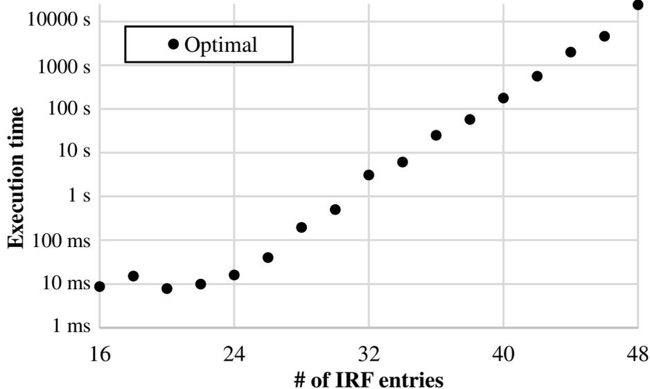
Figure 5: Execution time of the branch-and-bound algorithm to find the optimal selection.
