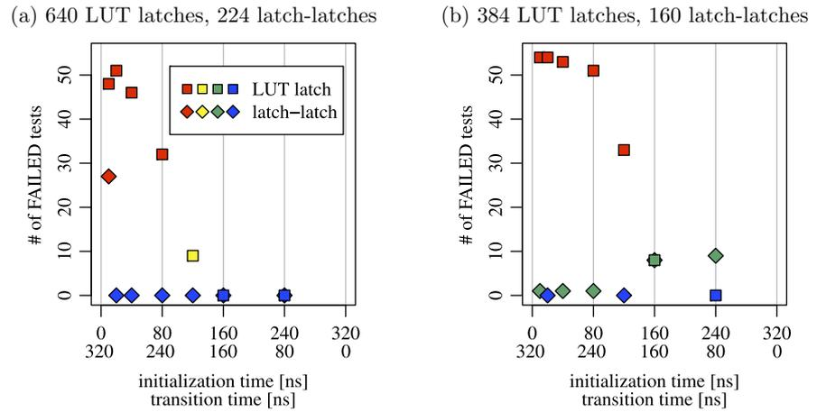
**Fig. 9.** The effect of the initialization time on the quality of randomness where the cycle time is fixed to 320 ns.
