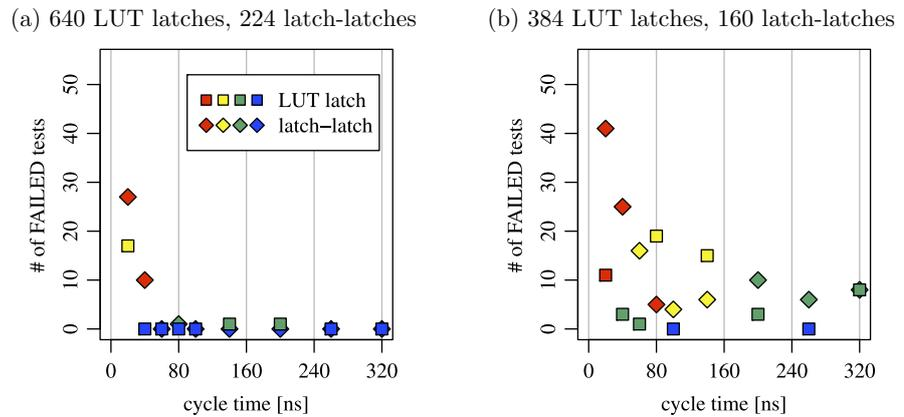
Fig. 7. The effect of the cycle time on the quality of randomness where  $t_i = t_l$ .
