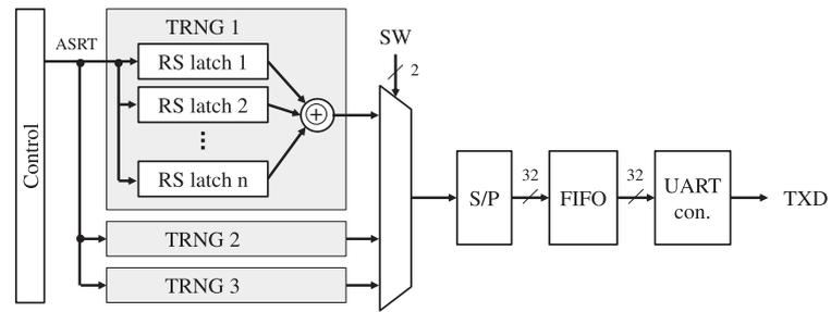
Fig. 5. Block diagram of the evaluation system.
