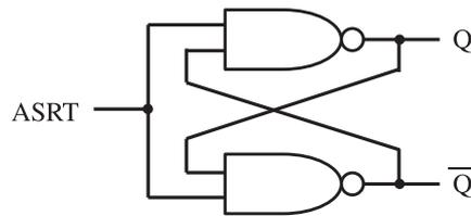
Fig. 1. A TRNG element based on the metastability of an RS latch.
