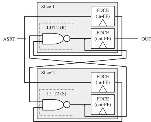
Fig. 2. An LUT latch, a composition of RS latch proposed by Hata and Ichikawa [6].
