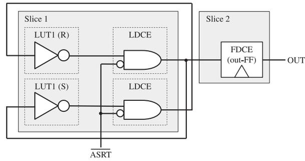
**Fig. 3.** Proposed latch-latch composition of RS latch.
