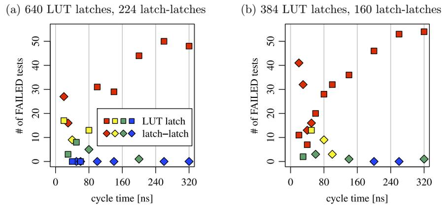
**Fig. 8.** The effect of the cycle time on the quality of randomness where  $t_i$  is fixed to 10 ns.
