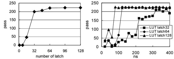
(a) The effect of the number of LUT latch. (b) The effect of sampling cycle.
